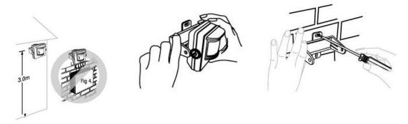
Select required location; position 3-4 metres above ground away from trees, direct sources of heat and direct sunlight.Remove LMDT-810 from base. Using base as a template, mark and drill 4 suitable holes.Secure base to wall using screws.Re-attach LMDT-810.Adjust angle and direction.
